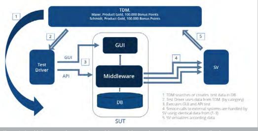
Figure 3: Combining a test data repository with a test driver and test-driven service virtualization
