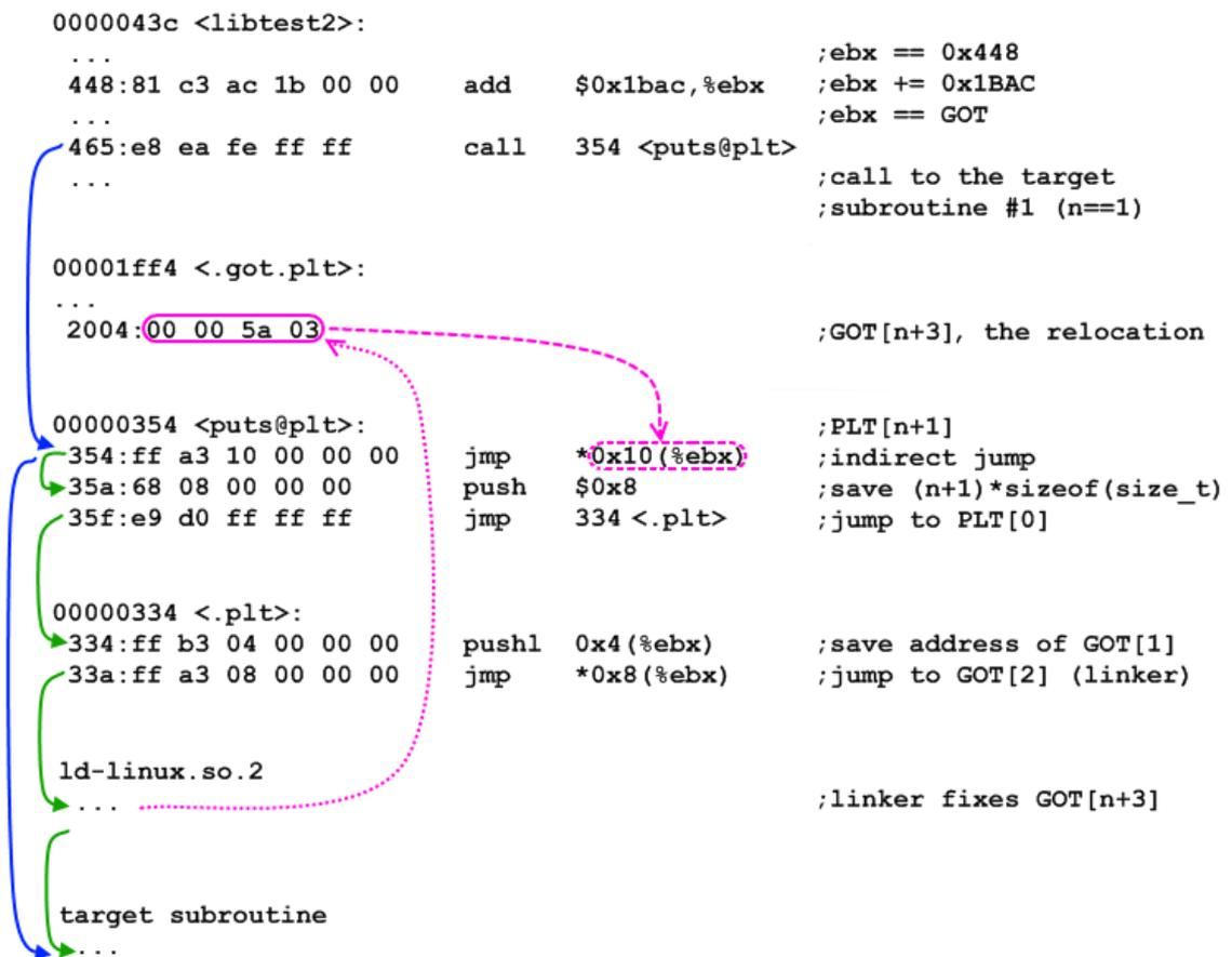
The relocation of R\_386\_JUMP\_SLOT type, which was used in the libtest2.so library, works in the described way. Other types of relocation refer to the static linking that is why we do not need them.
